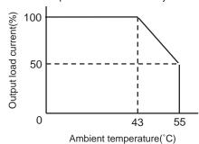
CP1W-32ER's maximum number of simultaneously ON output points is 24 (75%).
