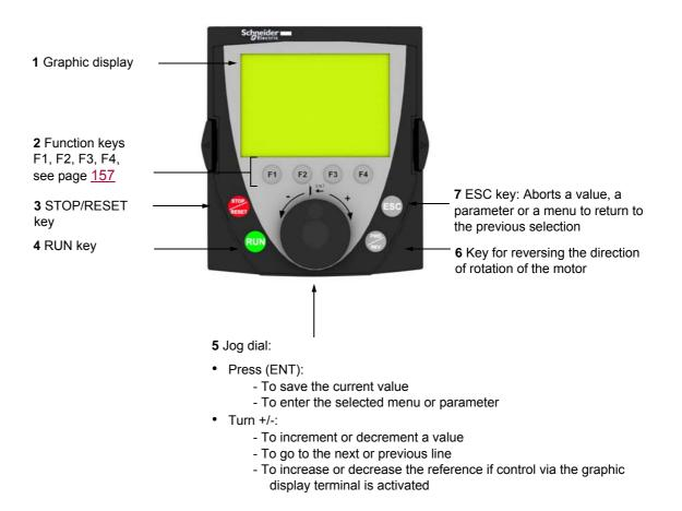
Note: Keys 3, 4, 5 and 6 can be used to control the drive directly, if control via the graphic display terminal is activated.
