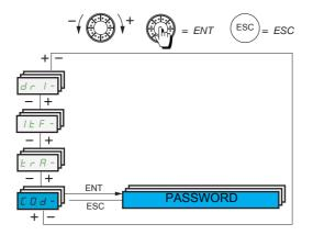
Enables the configuration to be protected with an access code or a password to be entered in order to access a protected configuration.
