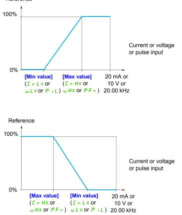
For +/- bidirectional inputs, the min. and max. are relative to the absolute value, for example +/- 2 to 8 V.
