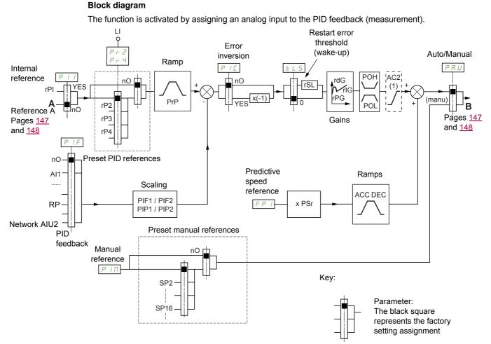
(1) Ramp AC2 is only active when the PID function starts up and during PID "wake-ups".
