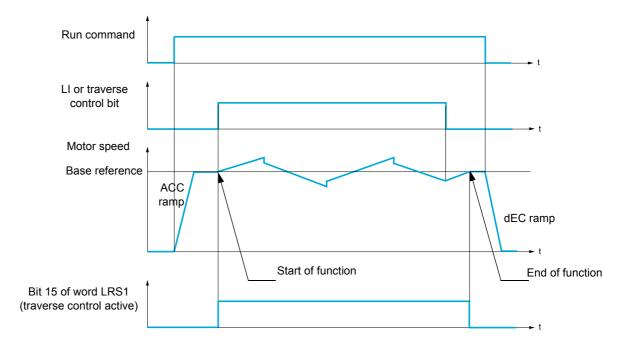
The function starts when the drive has reached its base reference and the traverse control command has been enabled.
