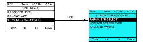
This can be used to configure the information displayed on the graphic display screen during operation.
