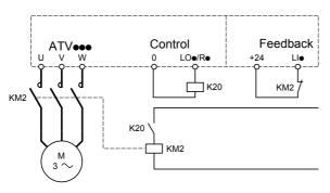
The [Out. contactor ass.] (  $\Box \ \Box \ \Box$  ) and [Output contact. fdbk] (  $\neg \ \Box \ R$ ) functions can be used individually or together.
