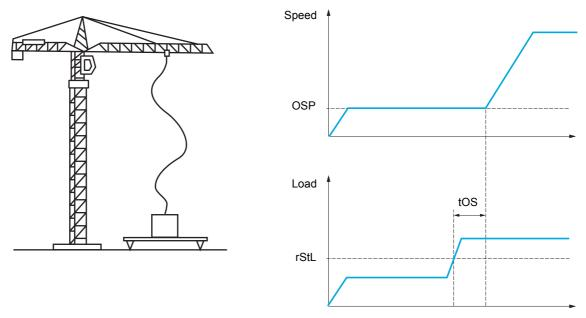
The speed step (OSP parameters) described on page 202 is used to measure the load. The effective measurement cycle will not be triggered until the load reaches the adjustable threshold [Rope slack trg level] (r 5 E L), which corresponds to the weight of the hook.
