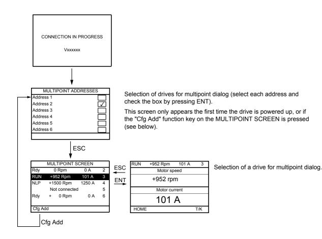
In multipoint mode, the command channel is not displayed. From left to right, the state, then the 2 selected parameters, and finally the drive address appear.
