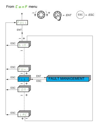
The parameters in the **[FAULT MANAGEMENT]** (*F L L -*) menu can only be modified when the drive is stopped and there is no run command, except for parameters with a O symbol in the code column, which can be modified with the drive running or stopped.
