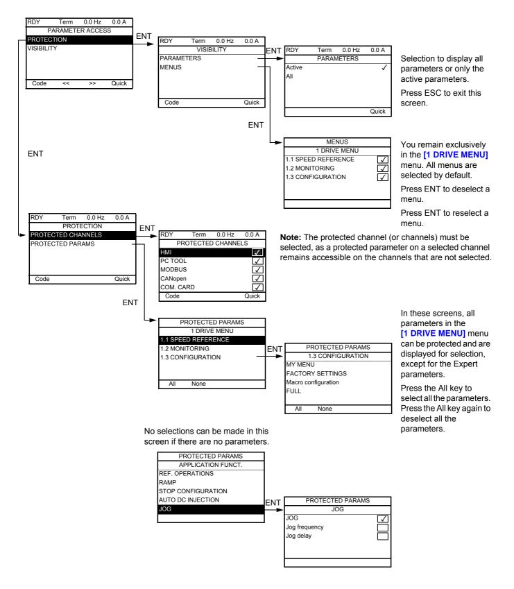
**Note:** The protected parameters are no longer accessible and are not, therefore, displayed for the selected channels.
