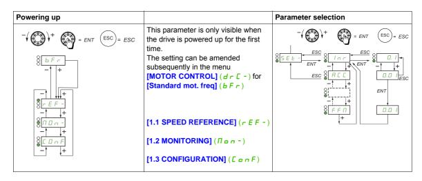
On the 7-segment display, a dash after menu and submenu codes is used to differentiate them from parameter codes.
